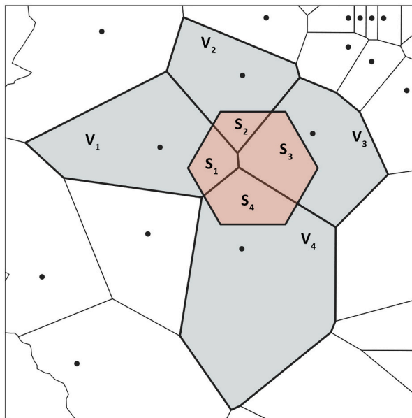
Fig. B.3. Convert the visitation frequency of tourists from cellphone towers to hexagons. Thiessen polygons are used to approximate the service areas of the cellphone towers.
